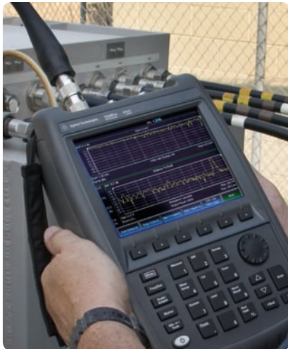
Perform and view return loss and distance to fault measurements at the same time
